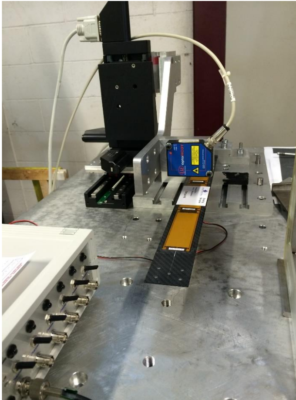
High voltage six-channel amplifier; one channel is used to give a positive voltage to the lower MFC patch close to the clamped section of a bending specimen
